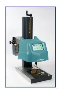
The P5000's design quickly adapts to part height (height up to 300mm/12 inches). Plus, it marks all types of materials up to a hardness of 62 HRC.
